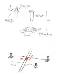
These markers shall be deployed 10m each side of an easily identifiable point of the pipe/ structure, in order to be able to detect small displacement using either top or lateral visual alignment or acoustic metrology using in this case, a saddle placed on the pipe.
